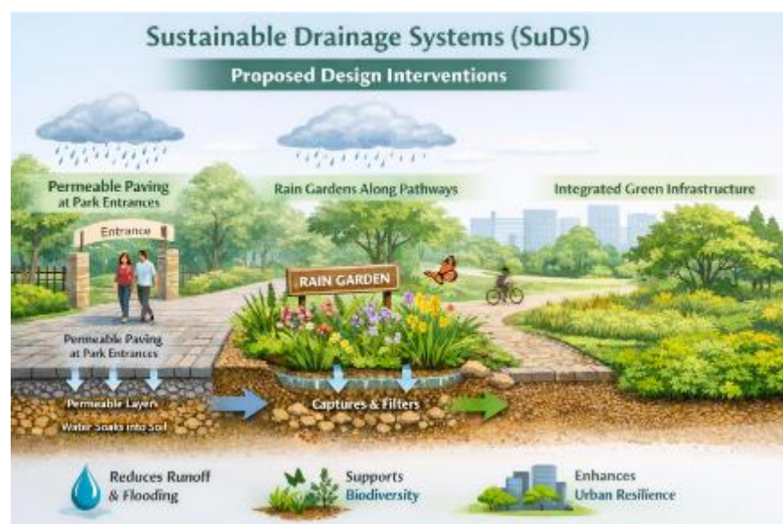
Figure 18. The Sustainable Drainage Systems (SuDS)
