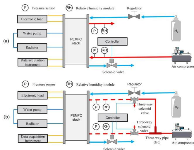
**Figure 1.** The original system (a) and Alternate air flow system (b) [1].
