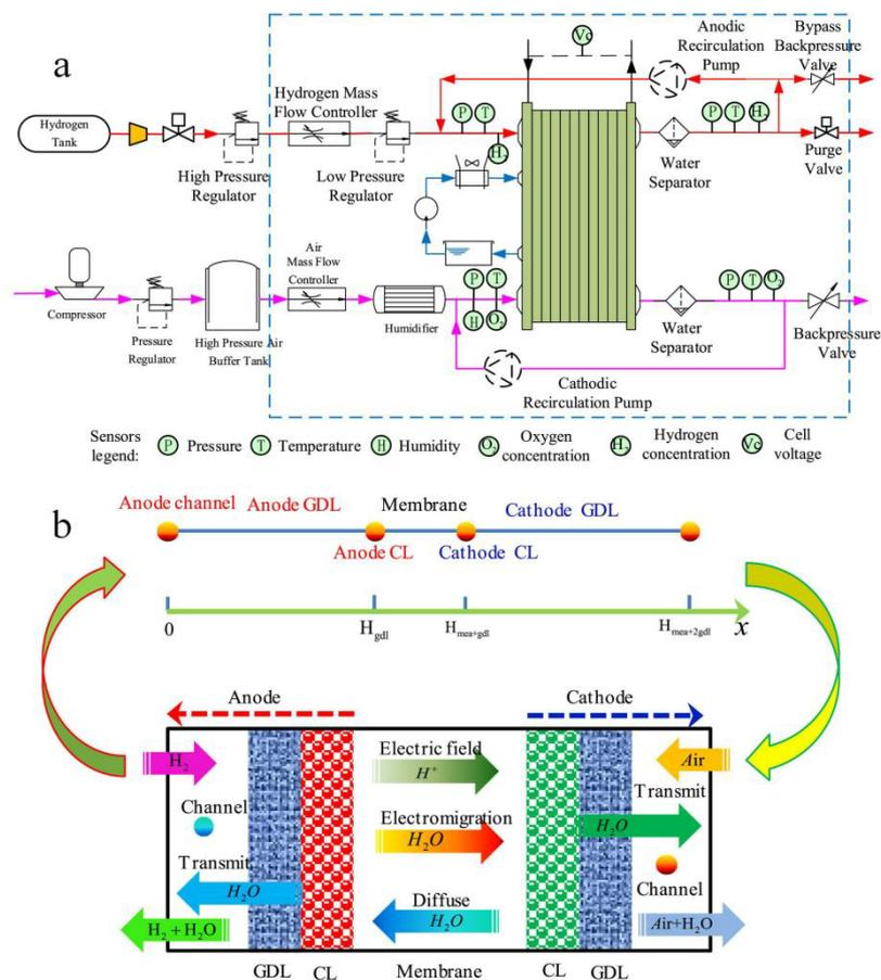
Figure 2. Schematic of PEM fuel cell dual recirculation system(a) and Schematic diagram of one-dimensional mechanism model (b) [6,9].
