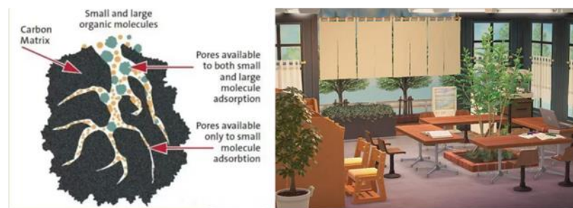
Figure 29. Proposed Air Quality Enhancement Measures: (Left) Adsorption Mechanism of Activated Charcoal and (Right) Integration of Indoor Greenery in Study Areas.
