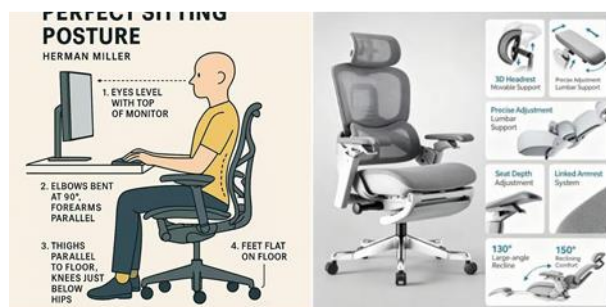
Figure 32. Principles of Ergonomic Sitting Posture (Left) and Key Adjustable Features of the Proposed Ergonomic Chairs (Right).
