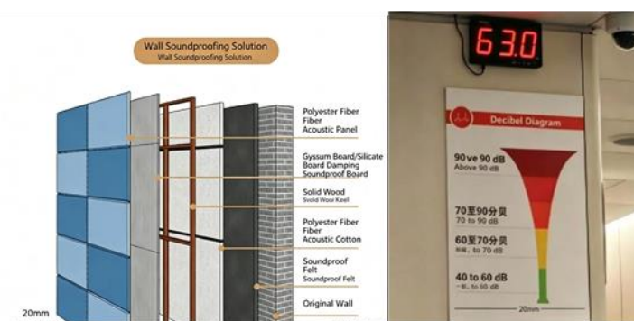
Figure 28. Proposed Noise Control Solutions: (Left) Structural Layers of Wall Soundproofing and (Right) Real-Time Decibel Monitoring System.
