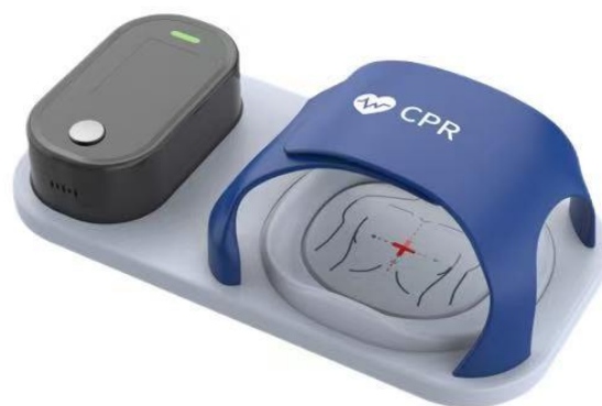
Figure 1. Appearance of the Self-Developed Flexible Wearable Chest Compression Assist Device Featuring a Liquid Silicone-Based Cushioning Substrate and Integrated Audio-Visual Feedback System.
